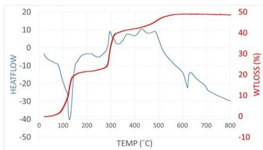
Fig 1. TGA and DSC curves for Sm-ZLD compound.
