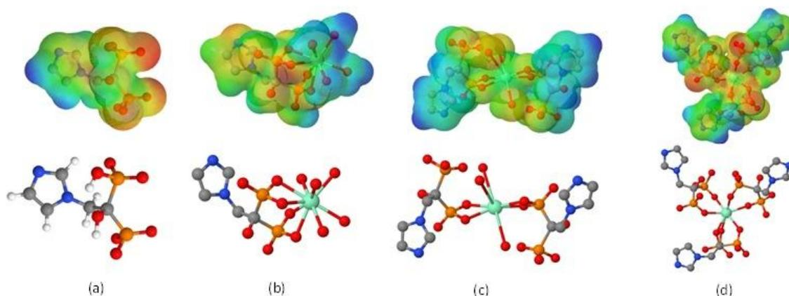
**Fig 2.** Schematic representation of optimized geometries and corresponding electrostatic potential energy maps of: (a) deprotonated ZLD ligand, (b)  $\text{Sm}(\text{ZLD})$ , (c)  $\text{Sm}(\text{ZLD})_2$  and (d)  $\text{Sm}(\text{ZLD})_3$ .
