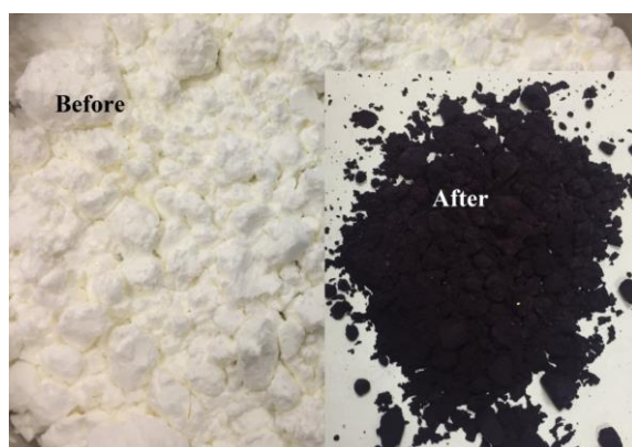
Fig 3. The starch powder before and after the stable iodine (I-127) trapping.
