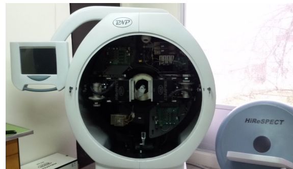
Fig 1. The developed dual head, high resolution animal SPECT system called HiReSPECT.
