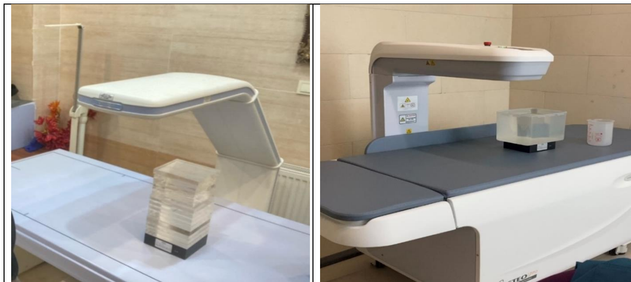
Figure 2. (Left) tissue-equivalent Plexiglas slabs placed above lumbar phantom, (Right) water tank placed above lumbar phantom
