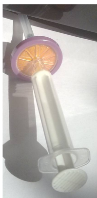
Fig 2. Syringe filter after use for filtering. Note significant amount of the tracer trapped in the filter (dark orange color of the filter).
