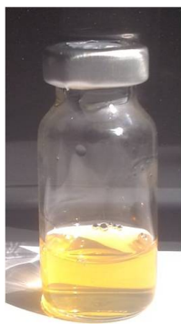
Fig 3. Filtered kit. Note reduction of the turbidity which is due to removal of the large particles.
