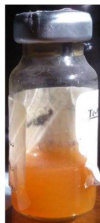
Fig 1. Labeled Tc-99m-Antimony Sulfide Colloid. Note the unusual turbidity of the prepared kit.
