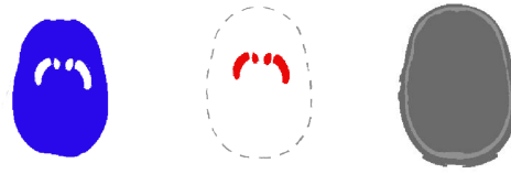
Fig 2. Striatal phantom: non-striatum background radioactivity distribution (left), striatum radioactivity distribution (centre) and the non-uniform attenuation map (right).
